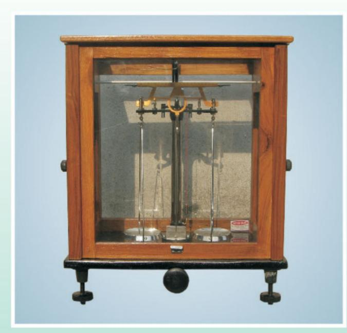
IBW' make TRIANGULAR BEAM ANAYTICAL BALANCE with Centre 'O' designed to withstand rough handling, suitable for use in Colleges, Universities, Industrial Laboratories and Research Laboratories.
